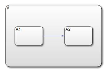
**6** Add the label E1 to the transition from state A1 to state A2 with this command:
