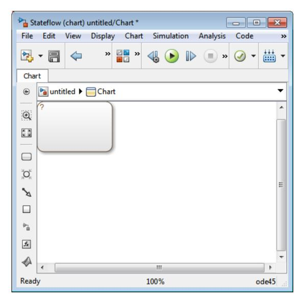
The constructor returns a handle to an API object for the newly created Stateflow object. Use this handle to display or change the object through its properties and methods.
