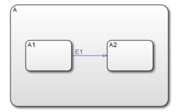
The state and transition labels in this chart are simple one-line labels. To enter more complex multiline labels, see "Enter Multiline Labels" on page 1-39. Labels for transitions also have a LabelPosition property you can use to move the labels to better locations.
